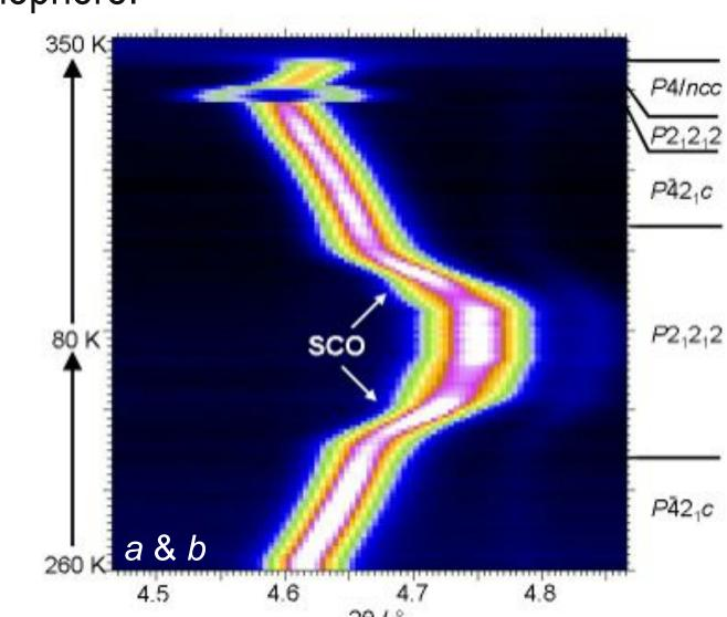
*In-situ* diffraction experiments at 1-BM revealed nine distinct structural phases within a complex sequence of phase transitions that describe both the SCO and the host-guest properties of SCOF-4.
