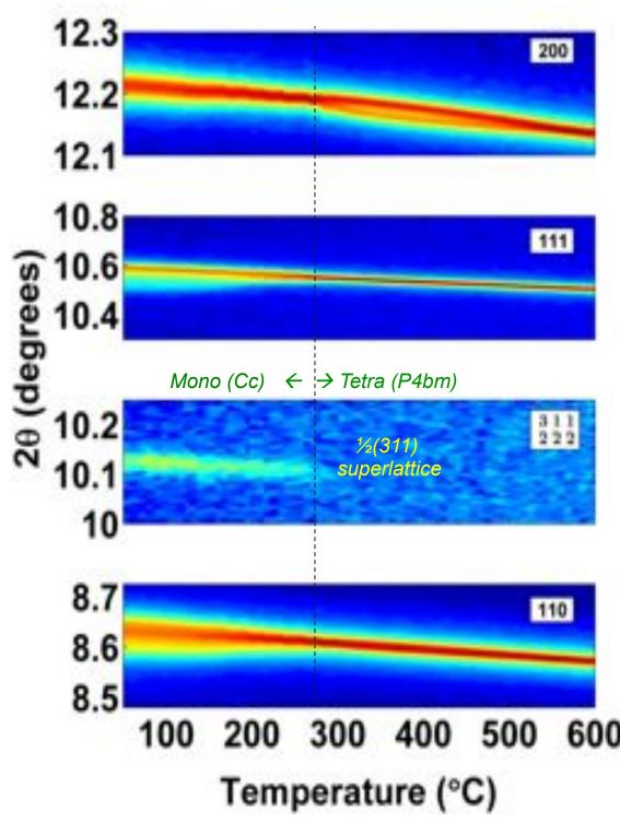
In-situ high temperature pXRD shows structural origins of depoling hysteresis in Na<sub>0.5</sub>Bi<sub>0.5</sub>TiO<sub>3</sub> piezoelectrics, and reveals new complexity in the parent ceramic material at ambient temperatures.<sup>2</sup>
